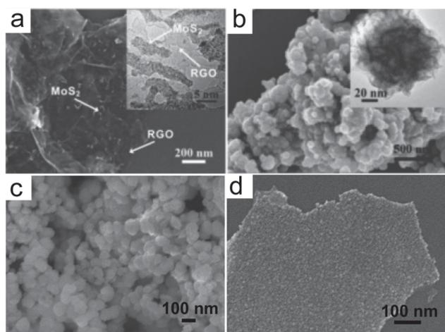
**Figure 1.** SEM and (inset) TEM images of a) the  $MoS_2$ /RGO hybrid and b) the free  $MoS_2$  particles; SEM images of c) pure CdS and d) 1 wt%-RGO/CdS nanocomposites samples. Reprinted with permission.<sup>[42,43]</sup> Copyright 2011, American Chemical Society.
