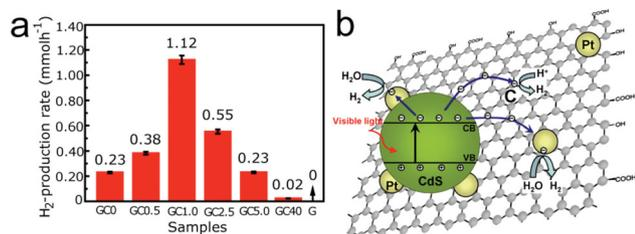
**Figure 3.** a) Comparison of the visible-light photocatalytic activity of samples GC0, GC0.5, GC1.0, GC2.5, GC5.0, GC40, and RGO for the  $\text{H}_2$  production using 10 vol% lactic acid aqueous solution as a sacrificial reagent and 0.5 wt% Pt as a cocatalyst. b) Schematic illustration of the charge separation and transfer in the RGO/CdS system under visible light. Reprinted with permission.<sup>[43]</sup> Copyright 2011, American Chemical Society.
