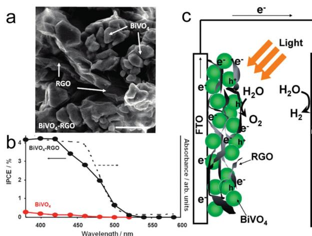
**Figure 5.** a) SEM image of BiVO<sub>4</sub>-RGO samples. Scale bars correspond to 600 nm. b) IPCE and diffuse reflectance spectra of BiVO<sub>4</sub> and BiVO<sub>4</sub>-RGO. c) Electron transport in a photoelectrochemical cell based on BiVO<sub>4</sub> and RGO. Reprinted with permission.<sup>[79]</sup> Copyright 2010, American Chemical Society.
