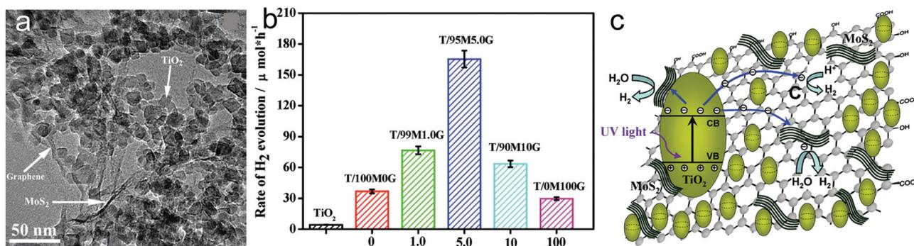
**Figure 10.** a) TEM images of T/95M5.0G composite. b) Photocatalytic H<sub>2</sub> evolution of TiO<sub>2</sub>/MG composites with different MoS<sub>2</sub> and RGO contents in the MG hybrid as cocatalyst under UV irradiation. c) Schematic illustration of the charge transfer in TiO<sub>2</sub>/MG composites. Reprinted with permission.<sup>[72]</sup> Copyright 2012, American Chemical Society.
