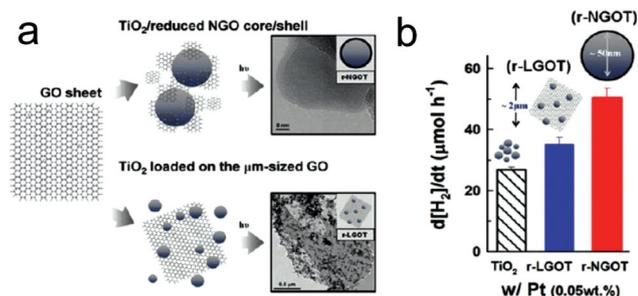
**Figure 2.** a) Illustration of the preparation procedure of r-NGOT and r-LGOT; b) Photocatalytic production of  $H_2$  in the aqueous suspension of  $TiO_2$ , r-LGOT, and r-NGOT in the presence of 0.05 wt% Pt ( $\lambda > 320$  nm). Reprinted with permission.<sup>[49]</sup> Copyright 2011, American Chemical Society.
